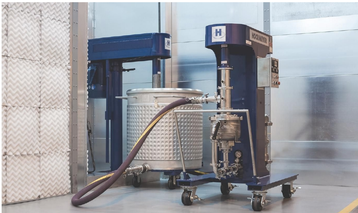
NexGen recirculation mill setup at Hockmeyer's Applications Laboratory.
