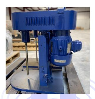
MOTOR 2 H.P.; 1800 RPM 3-PHASE; 60 CYCLE; 220/440 VOLTS Explosion Proof, Class 1, Group D
