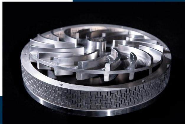
The clearance between the rotor's tips and the stator's inside diameter controls the discharge and shear rates.
